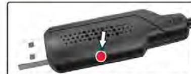
Red LED (Power LED) is solid on.
